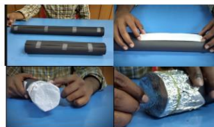
(a) Pinhole camera designed to measure size of large objects.
