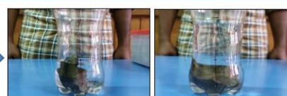
(a) Incorrect way to perform the task with the stone partly outside the water. (b) To start with larger initial amount of water so that the stone is completely submerged.
