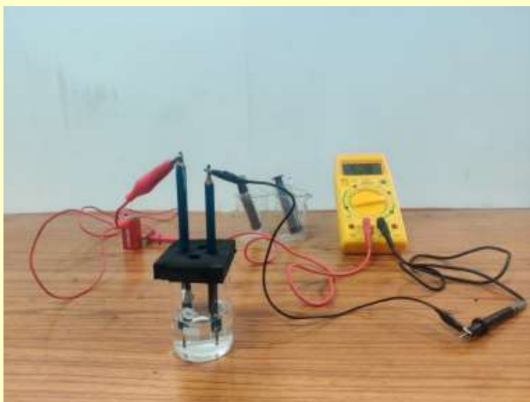
Figure 2 Electrical conductivity titration equipment with DC source
